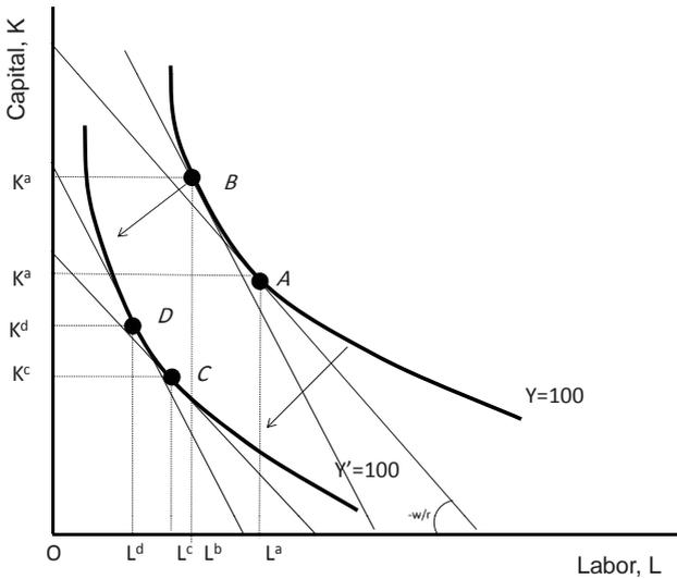
produce a given amount of output. Total factor productivity increases, when we move from the higher iso-cost curve to the lower curve at the left, because less capital and less labour are now required to produce the same amount of output.
